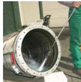
After cleaning the flame arrester and exchanging the bursting disc, the Q-Rohr is ready for use again.
