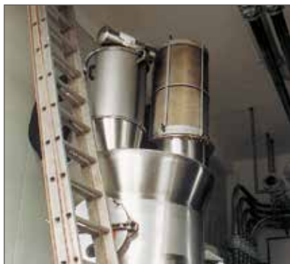
Q-Rohr installed in a milk powder factory
