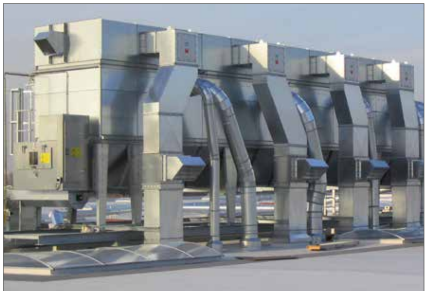
EX-GO-VENT explosion panels on filter system: Holtrop & Jansma, Netherlands
