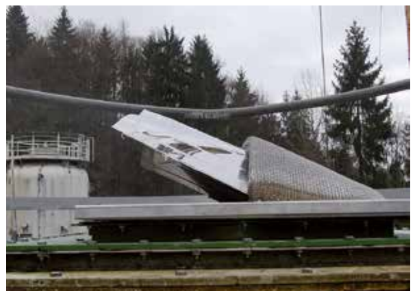
After occurred explosion venting: The TARGO-VENT technology limits the relief angle.
