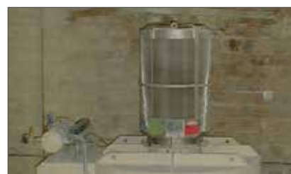
Explosion protection of a filter-cyclone combination in the fast food industry
