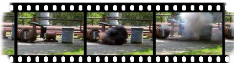
Explosion venting with the Q-Box II, no escaping flames
