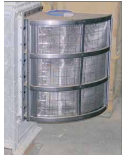
Q-Box on the foot of an elevator: economical solution compared with ducts
