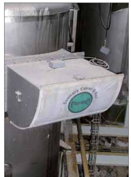
Q-Box application in the food industry with optional sanitary cover: Keeps the Q-Box clean!
